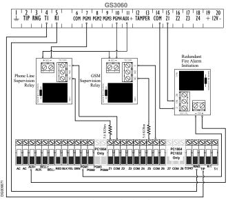
NOTE: Use EOL resistors in series with N.C. contacts of the relay.
