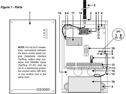
All circuits are classified for UL installations as Power Limited/Class II Power Limited except for the battery leads which are not power limited. Do not route any wiring over circuit boards. Maintain at least 1" (25.4mm) separation. A minimum 1/4" (6.4mm) of separation must be maintained at all points between Power Limited wiring and all other non-Power Limited wiring. Route wires as indicated above.
