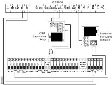
NOTE: Use EOL resistors in series with N.C. contacts of the relay
