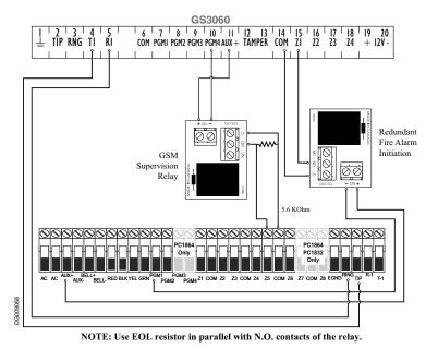
Figure 8 - Connection Details for GSM Supervision Relay, Phone Line Supervision and Redundant Fire Alarm Transmission
