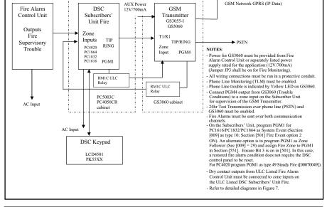
Figure 6b - DSC Subscribers' Unit Fire and GSM Transmitter Mounted Remotely
